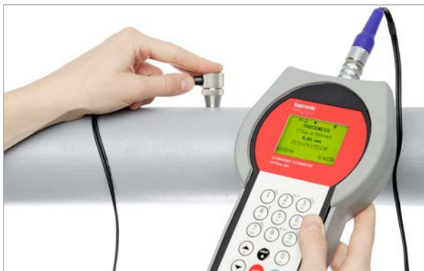
Wall thickness gauge NT with KATflow 200 in use
