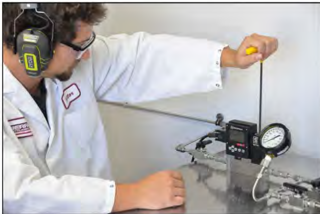
Mass Flow Controller Calibration: Valve Adjustment
