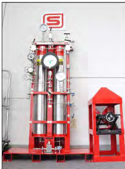
High-Pressure Accumulator Tank and Burst Test Manifold
