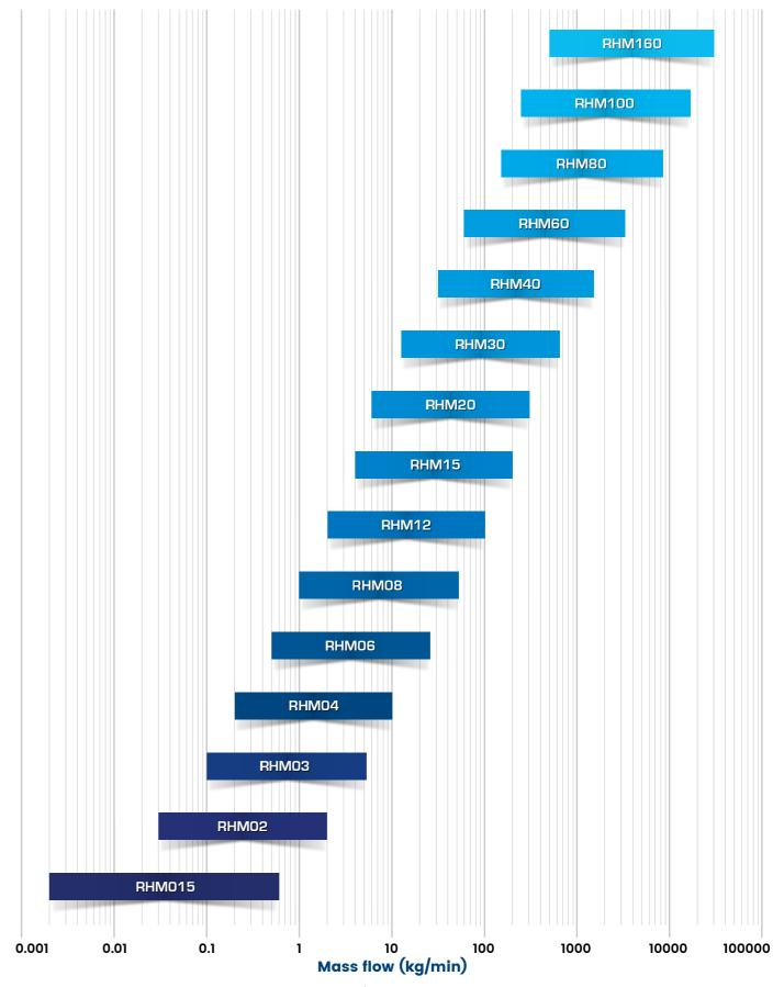
Flow rate chart depicts flow ranges for liquid applications at typical/common process pressure ratings. Flow ranges for meters with higher pressure ratings may vary. Gas flow ranges will depend upon pressure.
