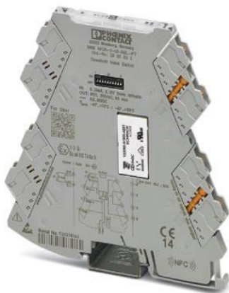
Figure 20 Limit value switch with changeover relay output for monitoring analog limit values from the sensor output. The sensor wash is activated at a mA value that corresponds to the limit value switch schedule with DIP switches activated. The relay closes or opens per user selection.
