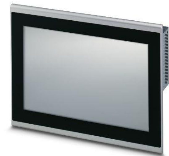
Figure 34 Panel mount external 7" touch display with connectivity of 4 sensors. Touch panel with 17.8 cm/7" TFT-display (Projective-capacitive (PCAP)), 1280 x 800 pixel(s) (WXGA), 16.7 million colors, Arm® Cortex®-A53, 4x 1.2 GHz, 2x USB host 2.0, 1 x Ethernet (10/100 Mbps), RJ45, Yocto/Linux and user software: Chromium Browser. (bus system: without)
