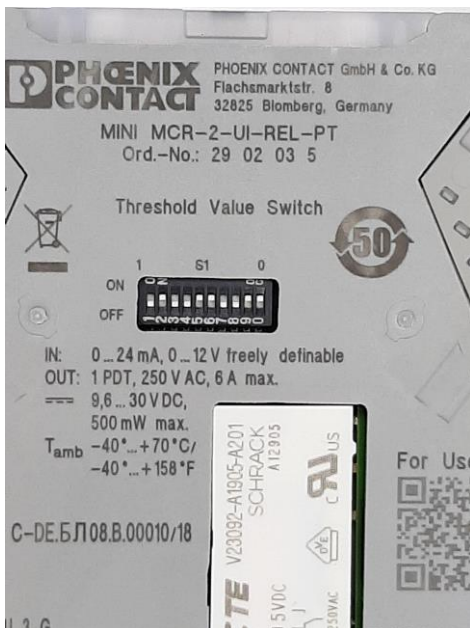
Figure 27 Physical DIP switch configuration for Low alarm functions. DIP switches 3, 5, 6, 9, 0 activated 'ON'
