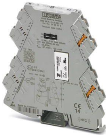
Figure 36 Limit value switch. Universally configurable limit value switch with PDT relay output and plug-in connection technology for switching analog limit values. Configurable via DIP switch or software. Push-in connection technology, standard configuration.
