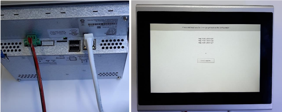
Figure 7 Cable connections to the external display and activation of configuration page during power up.
