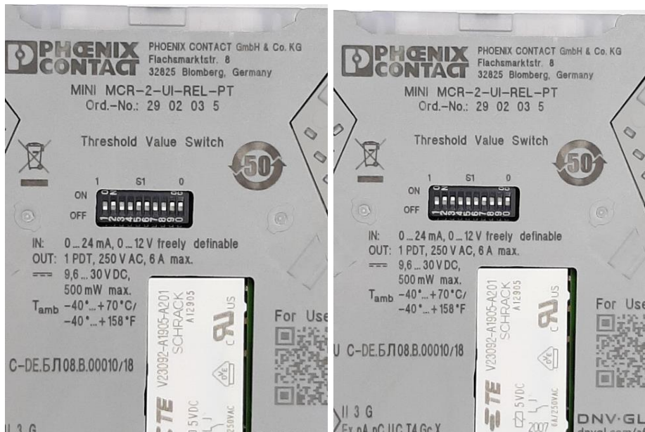
Figure 19 DIP switch configuration
